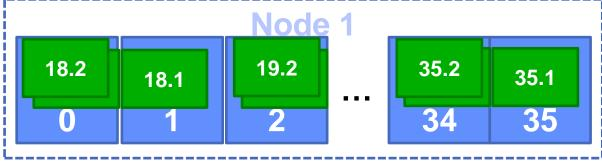
• In this case, the third thread is assigned to the same CPU as the master PE causing contention for resources.
