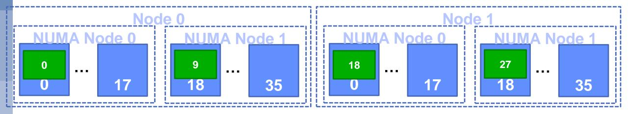
• PEs will be assigned to CPUs in the NUMA node in the standard order, e.g. 0-8,9-17, 18-26 and 27-35. However all CPUs within a NUMA node are essentially identical so there are no additional imbalance problems.
