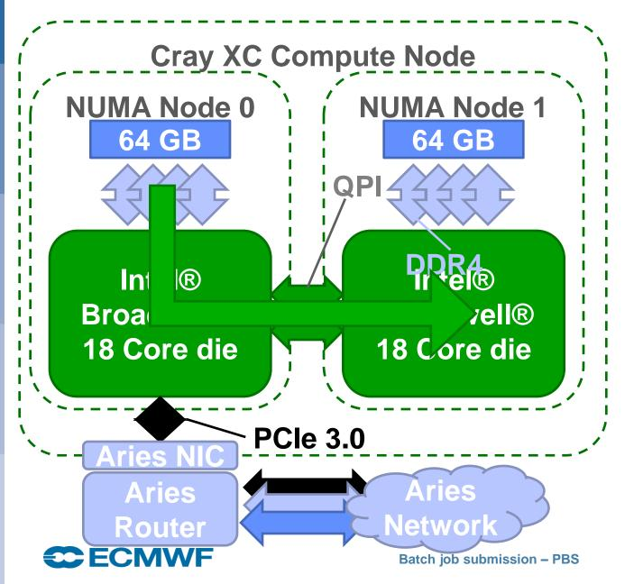
The design of the XC node means that CPUs accessing data stored on the other socket/die have to cross the QPI inter-processor bus
