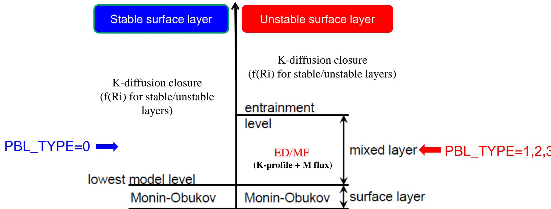
Figure 3.1 Schematic diagram of the different boundary layer regimes.
