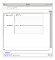
Now let us suppose that we want to compare the MSLP forecasts of the T1279\_ctl and T1279\_an experiments. Drop your 'mslp.mv' macro from folder 'T1279\_an' into the **Experiment 1** field, and drop your 'mslp.mv' macro from folder 'T1279\_ctl' into the **Experiment 2** field. Then click **Apply**.
